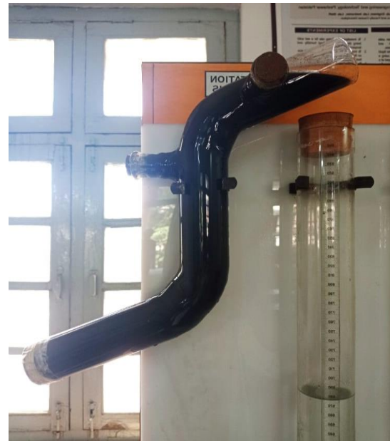
Fig. 2: Modified settling tank
